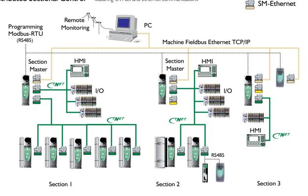
**Decentralized Control** — featuring CTSync drive-to-drive synchronization with less than 250µsec jitter
